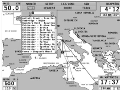
Once the desired port has been selected, the GEONAV-Multy will insert a waypoint in the port position and append the new leg to the existing route (if no route is available, the new waypoint will be connected to the boat's position).
