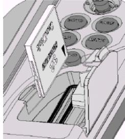
**NOTE:** Make sure of inserting the cartridge correctly. Should you try to insert the wrong side of the cartridge, full insertion into the slot is hampered. Any further attempt to force the cartridge into the slot may damage the cartridge or the **GEONAV-Multy's**. This kind of damage is not covered by the warranty.
