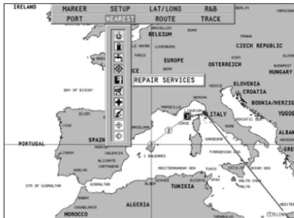
The GEONAV will insert a waypoint in the service selected, delete automatically the existing route then go back to Navigation mode and enable automatically the Autozoom function.
